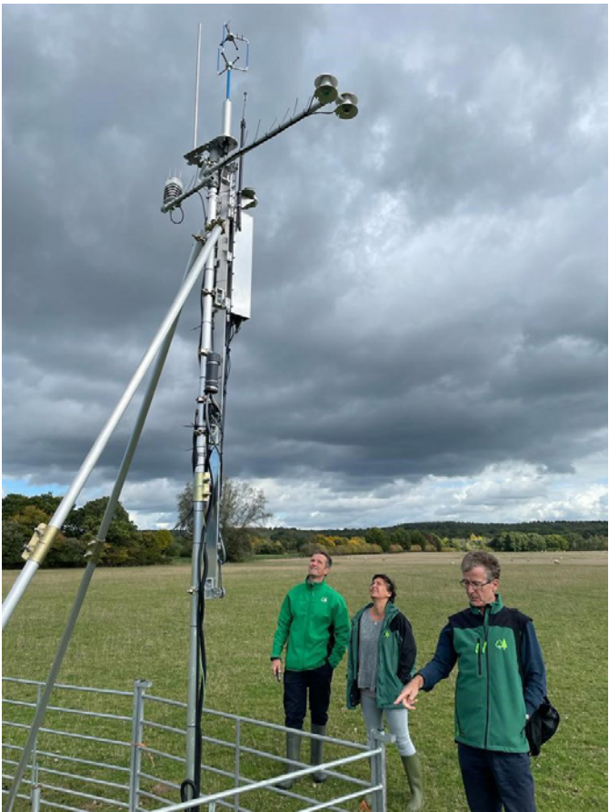
Above: Carbon flux tower at Alice Holt Forest field site. Credit: Kate Gannon
